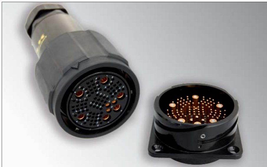
LKA 40/89: 80 pins size 18 for signal transmission, 6 coaxial pins, 3 pins size 12 for power. To obtain improved performance they may be used with many eurocable hybrid cables.
